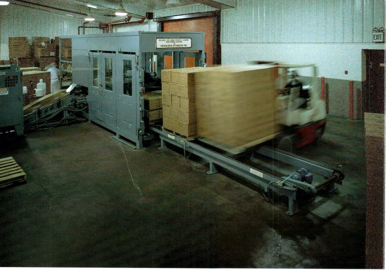
Production Automation (PAI) continues its pace-setting reputation for reliable high speed material handling with the Series 2600 palletizer. This floor level model consistently achieves speeds up to 50 cases per minute, depending on pattern and number of cases per load. Compare that to our competitors' claim of 20 cases per minute, and the benefits and cost savings of the Series 2600 are obvious.
