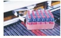
2. CASE TURNING: Turners retract with each case and require no adjustment for varying case weights. PAI's soft turn provides protection for the cartons and true. consistent turns.
