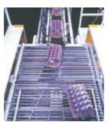
LINE DIVIDER: Cases are metered into the palletizer and divided into rows using PAI's smooth and efficient slat divider. The product is carried on urethane surfaced platens. Switching is accomplished by air operated UHMW shift-blocks, and diagonal movement of the platen is directed by use of a cam-roller on a hardened steel track.
