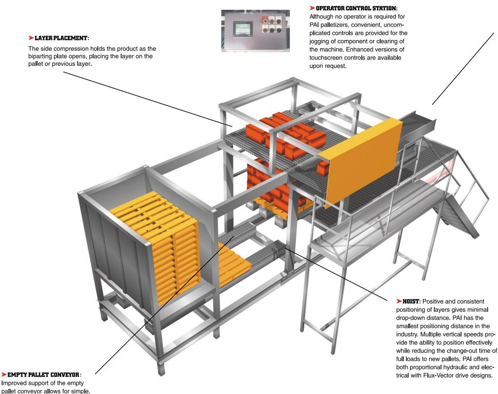
**CASE CONVEYOR:** Layer accumulating conveyors are designed (i.e. — stainless steel or low friction surfaces) for the characteristics of the product being handled. There are NO dangerous overhead rakes on these machines. Layers are conveyed into place without force of sweep-bars.
