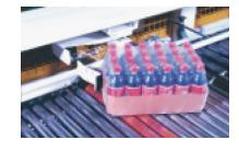
**CASE TURNING:** Turners retract with each case and require no adjustment for varying case weights. PAI's soft turn provides protection for the cartons and true, consistent turns.
