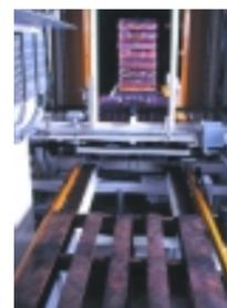
**7. EMPTY PALLET CONVEYOR:** Improved support of the empty pallet conveyor allows for simple, trouble-free handling of varying size and quality of pallets.
